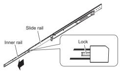
**2** Attach the inner rails to the right and left side of the server.
